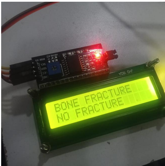
Fig5-Experimental Verification of LCD-Based Fracture Detection Output
