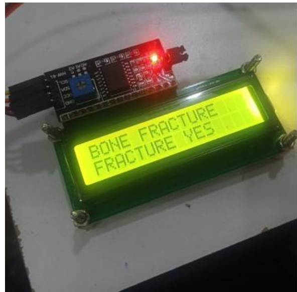
Fig5- Hardware Setup of LCD-Based Embedded System for Real-Time Status Display
